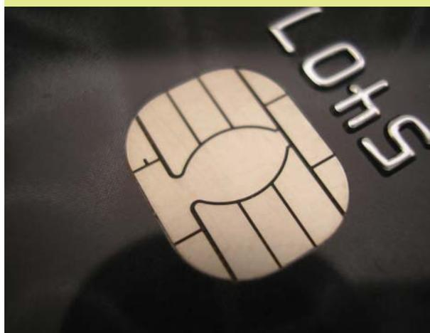
A chip embedded in a smart credit card.
